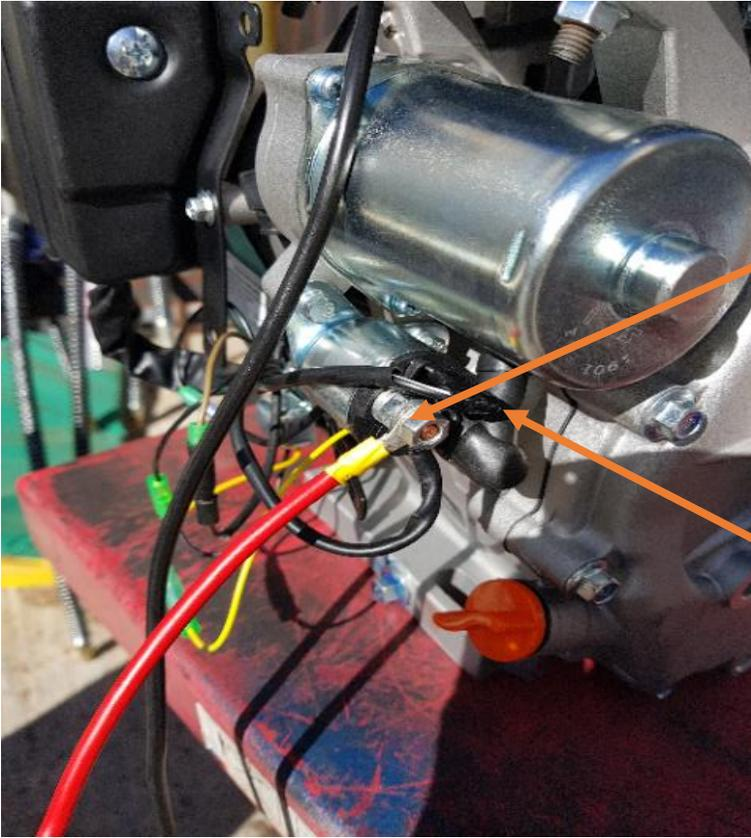
Red Battery Terminal, Place onto silver solenoid coil.
